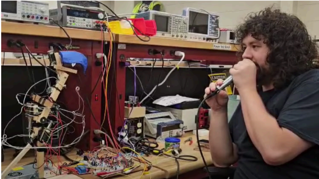
Figure 9.11: CAPER's mouth actuator being triggered by the VOX circuit
